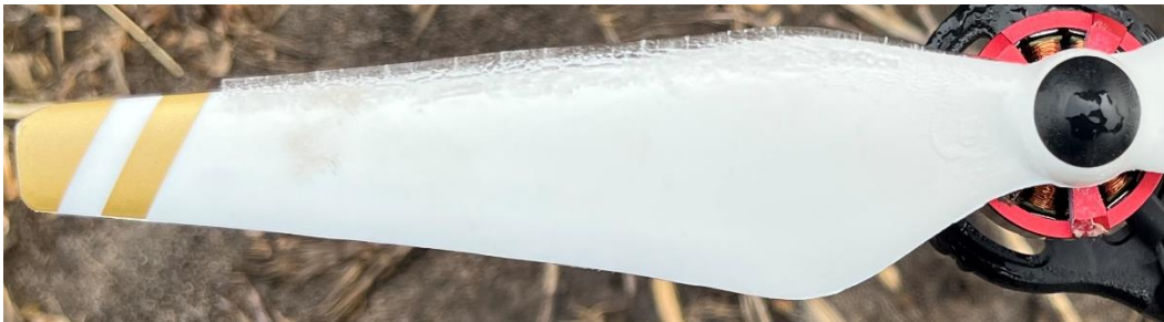
Figure 8. Ice formation on the suction side of a propeller.
