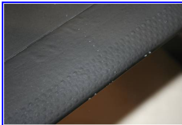
Figure 3: Finished leading edge with latex covering
