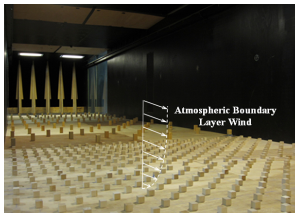
FIG. 1. AABL wind tunnel used for the present study.
