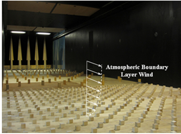
Fig. 1 Test section of the AABL wind tunnel
