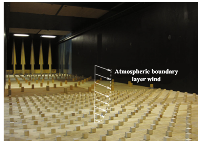
Fig. 1 Test section of the AABL tunnel used for the experimental study
