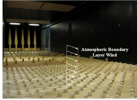
Fig. 1. The test section of the AABL wind tunnel.
