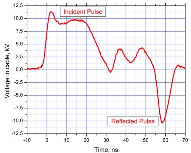
Figure 5. A typical high voltage driving signal calculated through the back current shunt measurements as a function of time ( t ) in nanoseconds.
