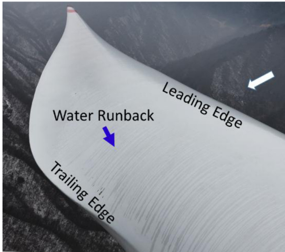
Fig. 1. A photo of the water runback behaviors taken at the beginning of a glaze icing process over the pressure-side blade surface of a 2 MW wind turbine.
