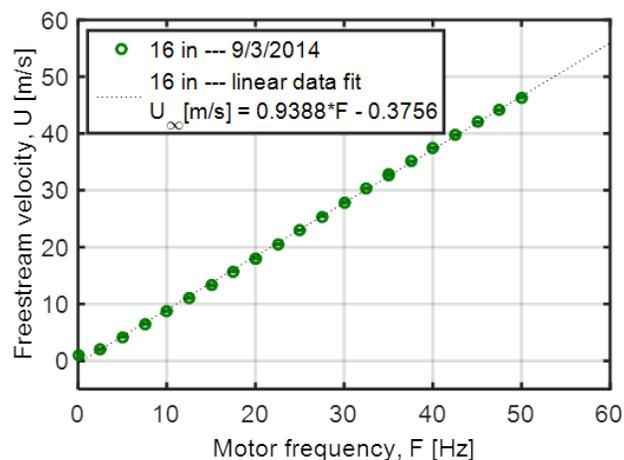
Figure 1. Wind tunnel air speed versus motor frequency setting.
