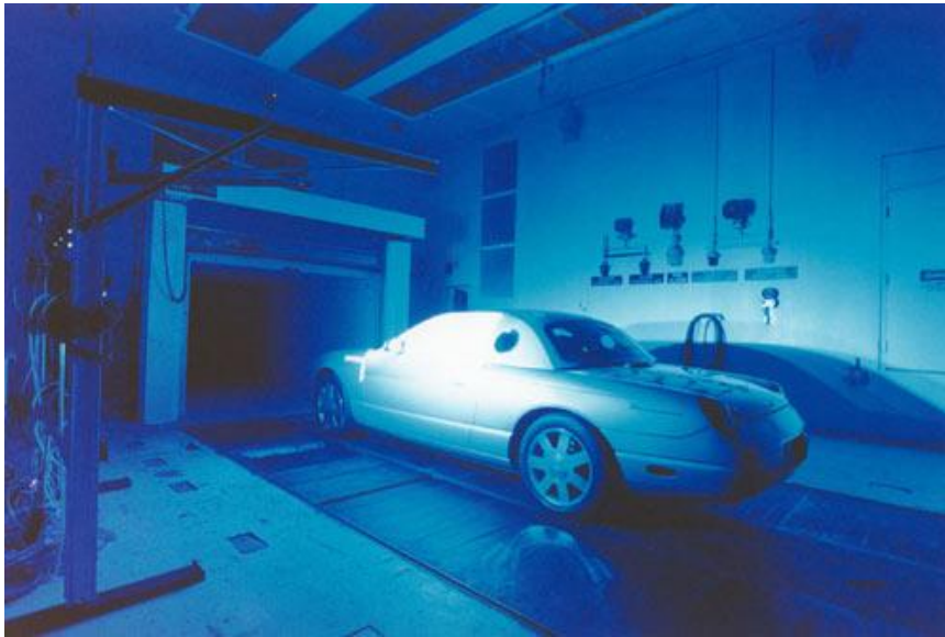
PSP measurements of a 2002 Ford Thunderbird
