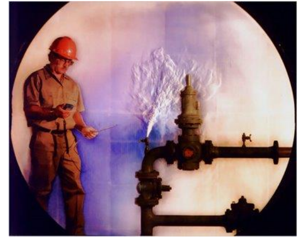
A gas leak
