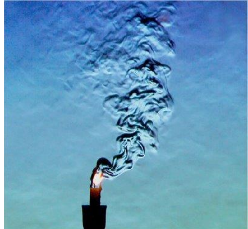
Schlieren image of a thermal plume of a burning candle
