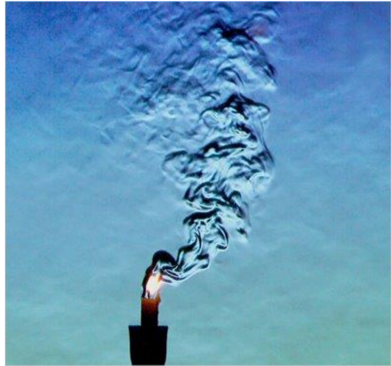
Schlieren image of a thermal plume of a burning candle
