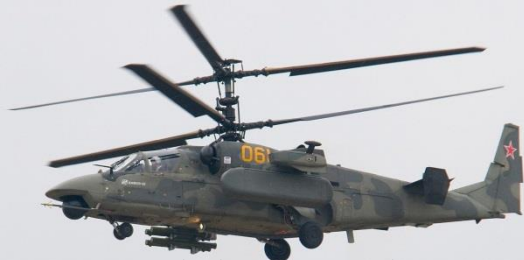
Soviet Ka-2 helicopter with counter-rotating rotors
