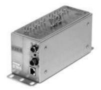
Tubes are connected from pressure taps in the walls of the wind tunnel to the ports on the DSA. One of the ports on the DSA is labeled "Reference." The pressures that you will read in your data files will be pressure differentials as follows:
