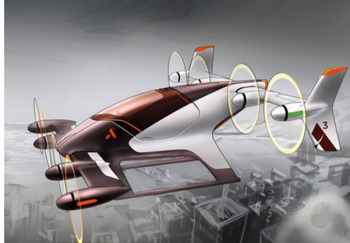
Fig. 1 Airbus Vahana with tandem tilt-wing configuration during the cruise phase [19].
