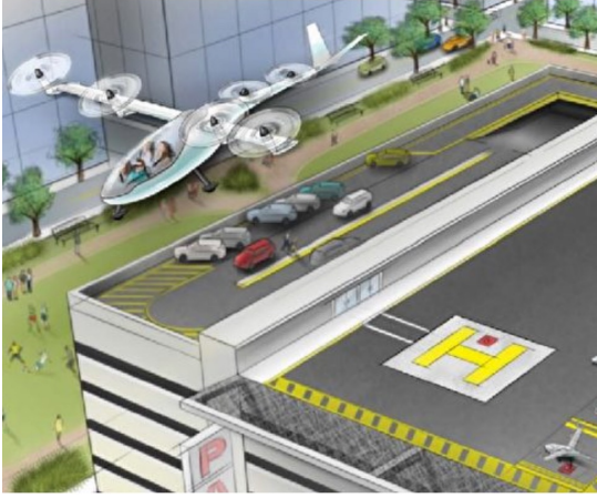
Fig. 2. Vertiport with single landing pad [2]
