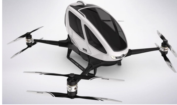
Figure 1. EHang 184: coaxial multi-rotor eVTOL air taxi with X8-configuration 15
