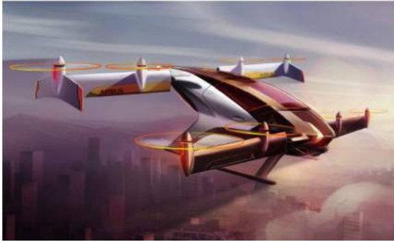
Fig. 4. Airbus Vahana: Tandem tilt-wing configuration during the descent phase [7]
