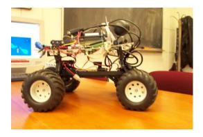
Figure 2. Vehicle with PC-104 computer.
