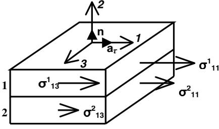
Fig. 1: Components of the stress tensor that are discontinuous across the interface  $\Sigma$  and therefore contribute to  $\mathbf{X}_n$ , the driving force for IR.
