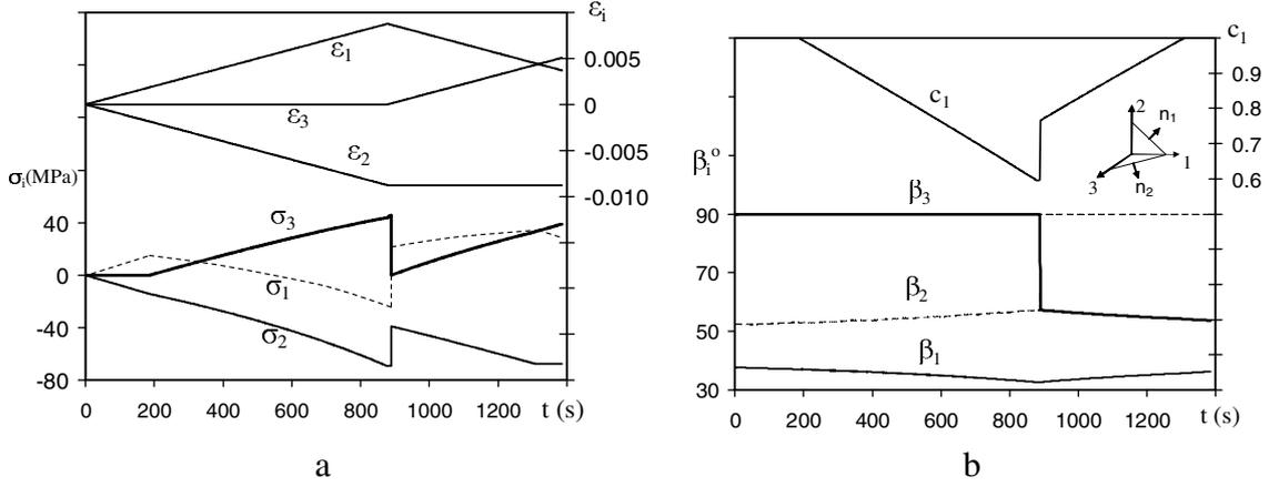
Fig. 3: (a) Prescribed strain history and the corresponding stresses, and (b) the evolution of the volume fraction  $c_1$  and the direction angles,  $\beta_i$ , between  $\mathbf{n}$  and the coordinate axes for a tetragonal-orthorhombic PT. The jump in the normal is accompanied by a jump in volume fraction (reverse PT) and all macroscopic stresses.
