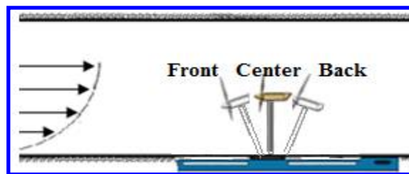
Figure 3: Illustration of turbine's oscillation in pitch motion.
