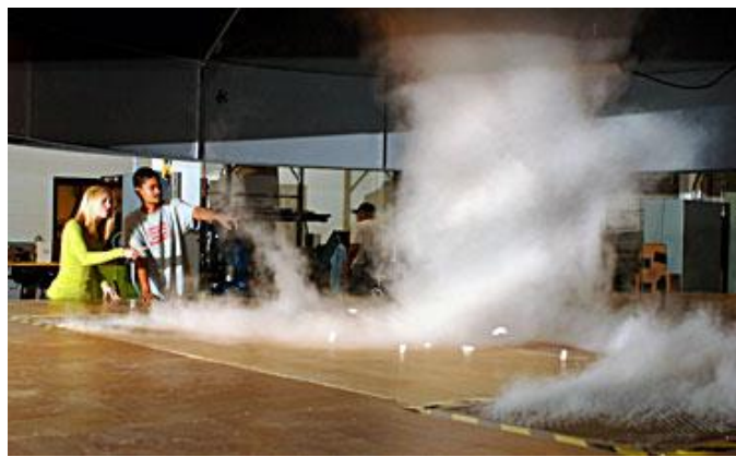
The world largest moving Tornado/Microburst Simulator D_{\text{tornado}} = 0.5 \text{ m} \sim 2.0 \text{ m}
