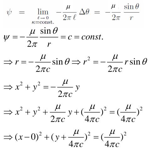
Streamlines are circles centerd on the *y*-axis a distance  $-\frac{\mu}{4\pi\psi}$  from the *x*-axis with a radius of  $\left|\frac{\mu}{4\pi\psi}\right|$ . All circles pass through the origin.
