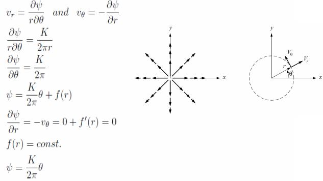
Since the source strength, K is a constant,  $\psi$  constant lines are radial lines.
