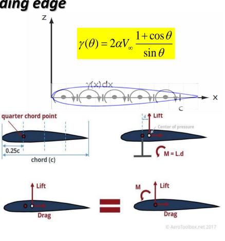
$\alpha = 0 \implies C_{M,LE} = 0$   $\alpha = 5^{\circ} \implies C_{M,LE} = 0.11$  $\alpha = 10^{\circ} \implies C_{M,LE} = 0.22$
