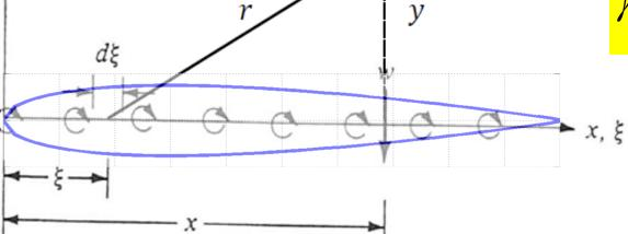
The Kutta-Joukowski Lift Theorem states the lift per unit length of an airfoil is equal to the density (ρ) of the air times the strength of the rotation (Γ) times the velocity (V) of the air.
