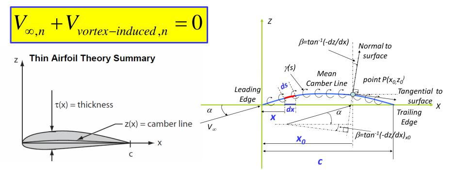
• To force the mean camber line to be a streamline, the sum of all velocity components normal to the mcl must be equal to zero.
