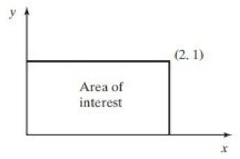
**Problem#3:** Given an incompressible, steady flow, where the flow velocity is  $\vec{V} = (x^2y - xy^2)\hat{i} + (\frac{y^3}{3} - xy^2)\hat{j}$
