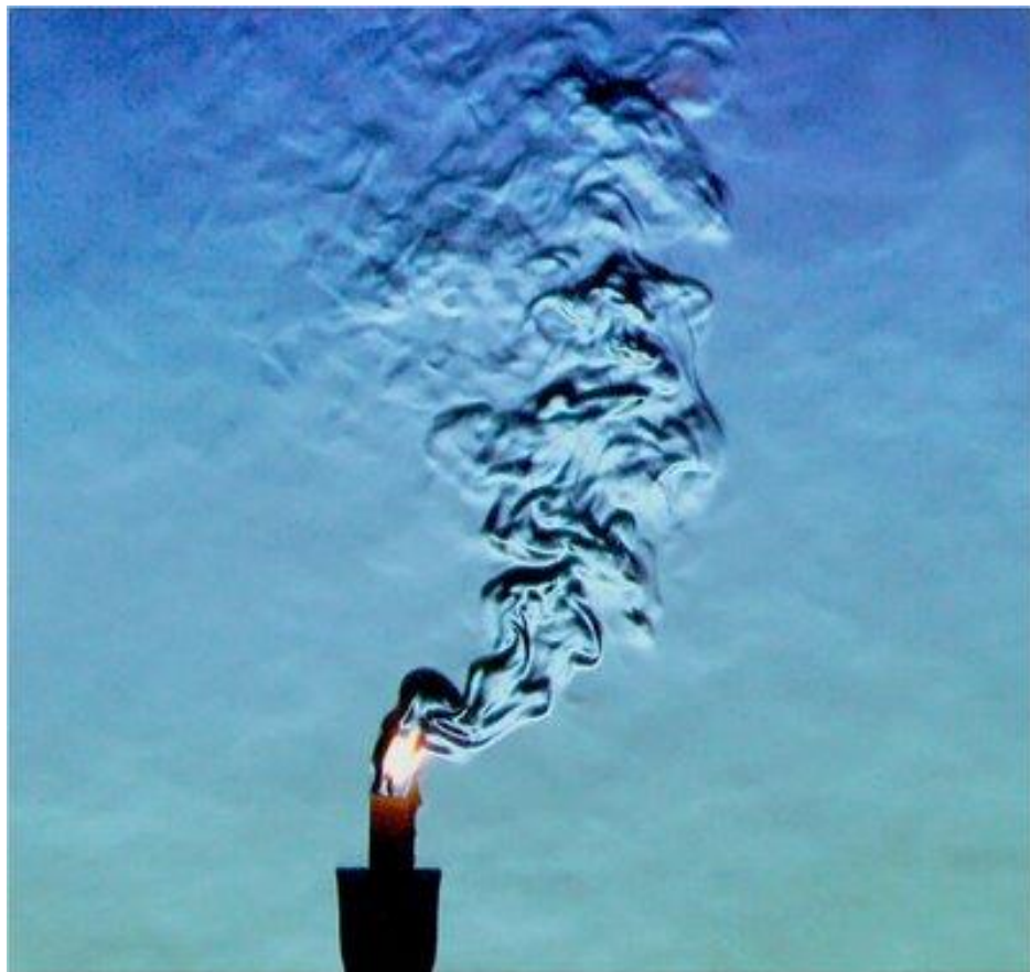
Schlieren imaging result of a thermal plume above a burning candle
