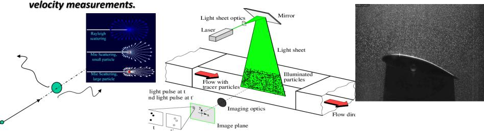
Molecular-based techniques usually leverage lased-induced photoluminescence of the tracer molecules to measure multiple flow properties (velocity, temperature, pressure, concentration...).
