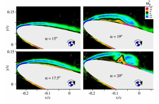
Boundary layer resolved vorticity measurements have revealed the flow physics at the onset of the separation process, and its spatial and temporal scales.
