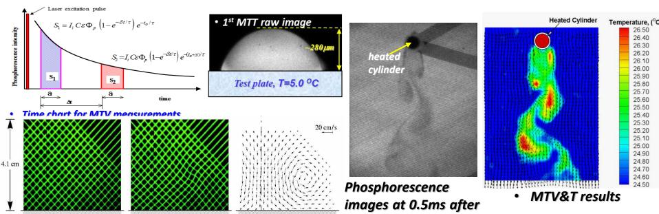
Molecule-based techniques, - Molecular Tagging measurements
