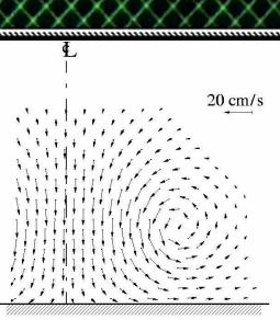
The velocity field derived using a spatial correlation procedure
