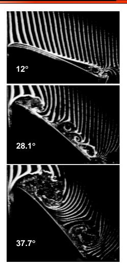
NACA-0012 airfoil pitching to high angle of attack
