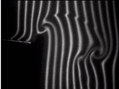
Flow visualization of the vortex shedding from the trailing edge of an oscillating airfoil (Bohl et al. 2002)
