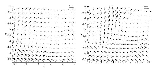
Two instantaneous realizations showing the large cycle-to-cycle variability of the flow field.
