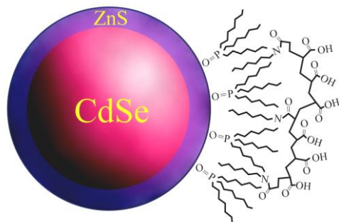
The structure of a (CdSe)ZnS quantum dot
